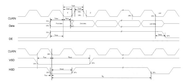
**Input Clock and Data Timing Diagram**
