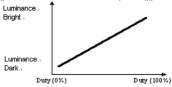
2. ADJ signal =  $0 \sim 5.0V$ , operation frequency :  $200Hz\sim20KHz$
