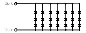
Note(6) When LCM is operated over 60°C ambient temperature, the IAK of the LED backlight should be adjusted to 105 mA max
